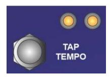
If GKA is enabled the left LED will turn ON If GKB is enabled the right LED will turn ON
