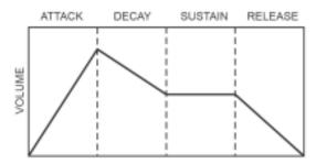
This diagram shows a typical ADSR envelope of a note played. The ENVELOPER effect allows you to change the volume during these four stages. For example if you remove the initial attack you get a smooth bow-like sound.
