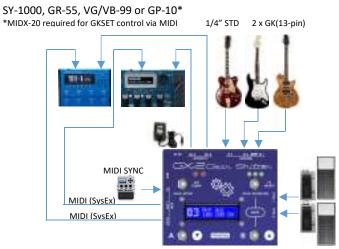
Never connect or disconnect GK connectors while power is ON
